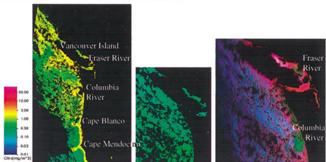
Fig. 4. Standard OCC product, left, standard SST product, center, and water pixel classification result, right, for the Vancouver Island Canada, 1 May, 1997.
